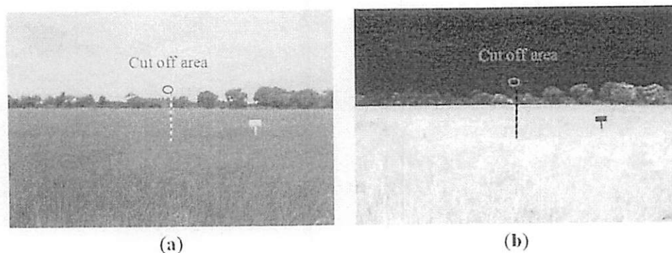
Figure 15. Cut off area (red circle) in (a) RGB and (b) modified filtered excess green images.
