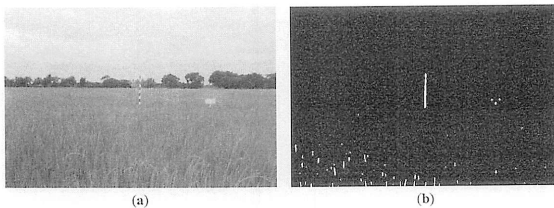
Figure 20. Comparison between (a) RGB and (b) resultant binary images using proposed method with excess green feature on 19 July 2012.
