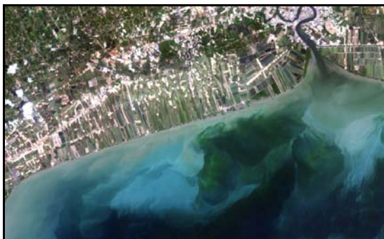
Fig. 3. Shows the images from Landsat-8 upon False Color composite: 4, 3, 2. It is difficult to separate the oil stained area from the sea water with dregs.
