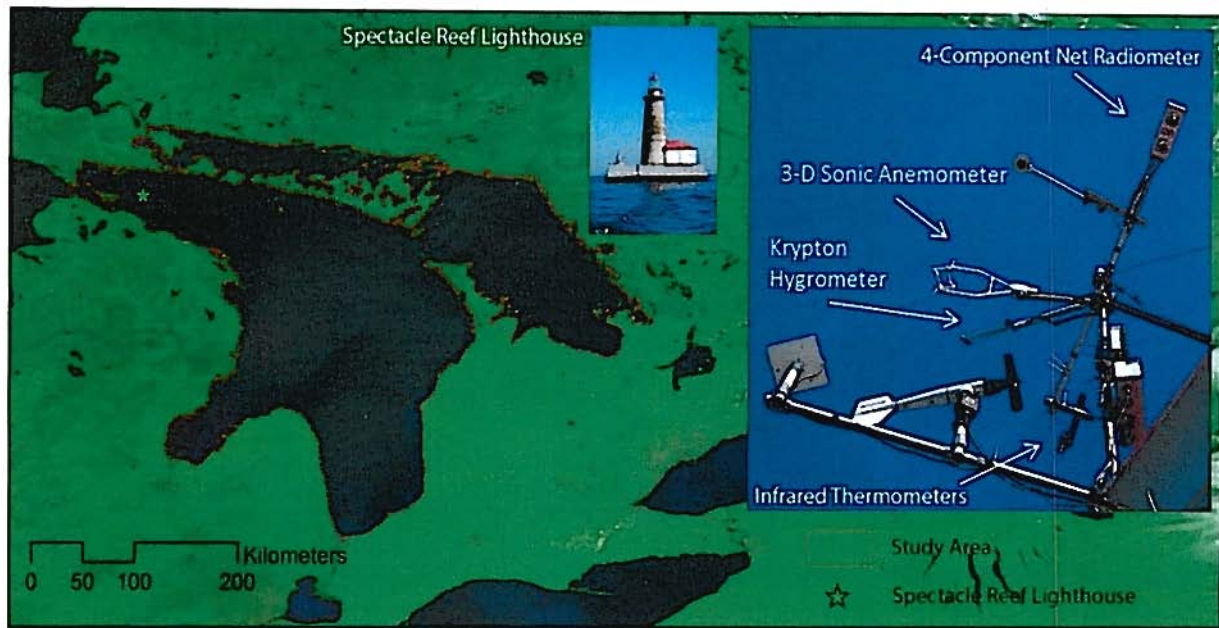
Figure 1. Satellite mosaic images from MODerate Resolution Imaging Spectroradiometer (MODIS) showing the study area and location of Spectacle Reef Lighthouse with the meteorological station located on the top
