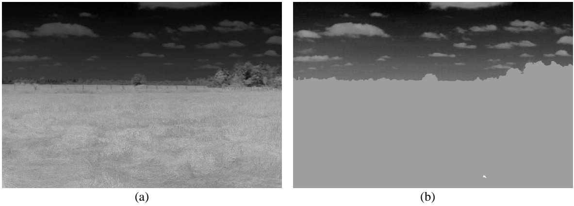
(a) (b) Figure 4. Normalized red minus blue image (a) and sky-masked normalized red minus blue image (b)
