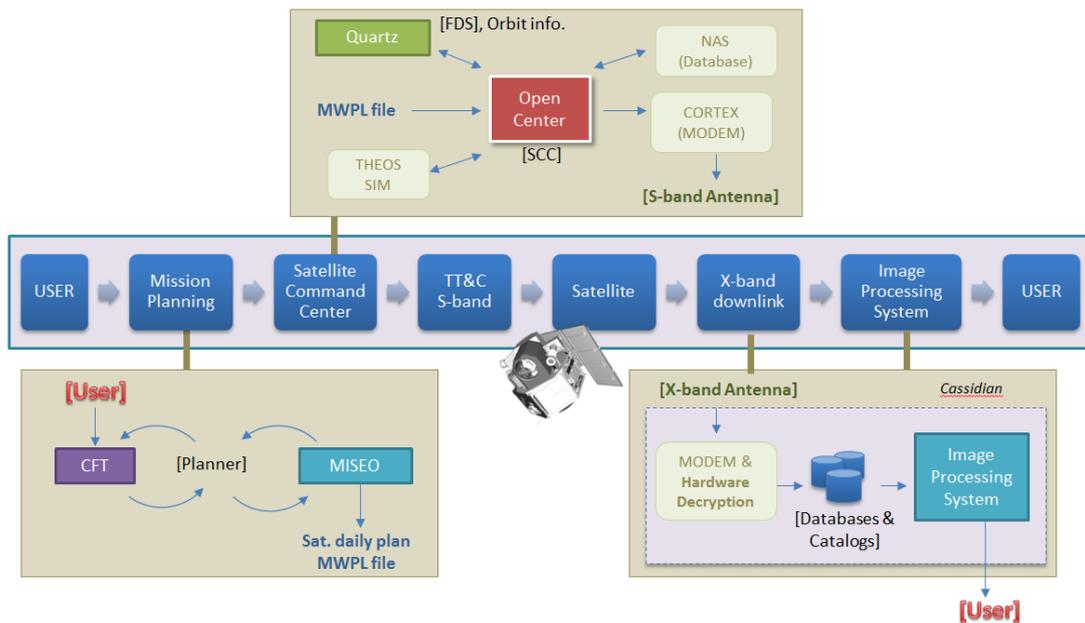
Figure 1: Current workflow for Thaichote ground segment operation.
