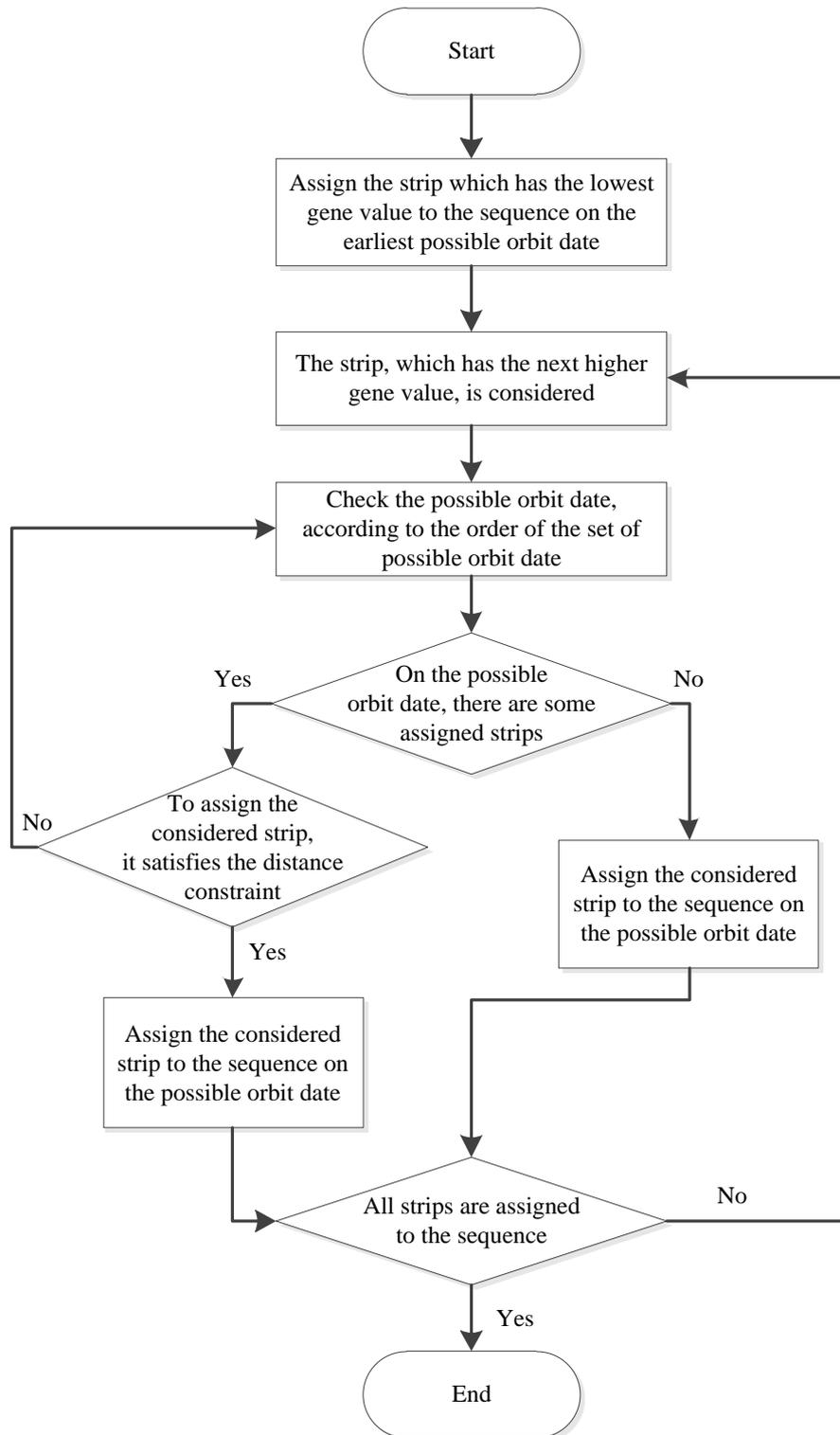
Figure 5: Flowchart of decoding step
