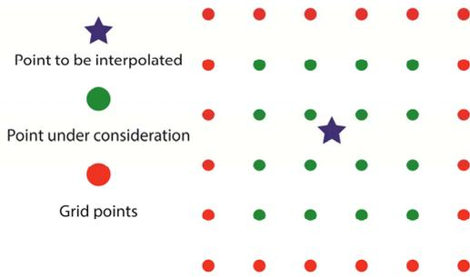
Fig. 2. The interpolated value (blue star) is a weighted sum of the 4x4 nearest pixels or 16 grid points (green dots).
